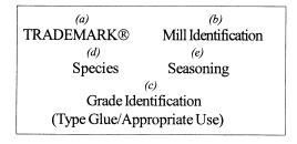
Grade stamps on glued lumber include all the information indicated for visually graded lumber. In addition, the grade stamp includes a designation or abbreviation indicating the type of glue joint and appropriate use. Examples include "Stud Use Only", "Vertical Use Only", "Certified End Joint", "Certified Exterior Joints", "Heat Resistant Adhesive", and "Non-heat Resistant Adhesive".
